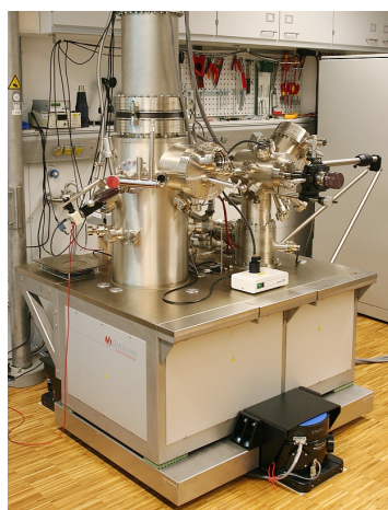
65 Series STACIS® Floor Platform supporting an Omicron Multiprobe Scanning Tunneling Microscope (STM) with nanometer scale resolution at the Max Planck Institute in Dresden, Germany.
