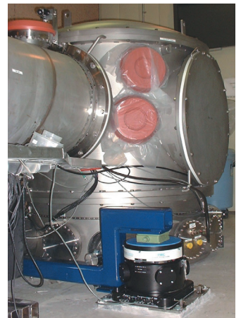
STACIS® supporting the end chambers of a prototype LIGO interferometer at the California Institute of Technology. These are the most precise instruments ever made – capable of measuring distances of less than 10 -18 m.
